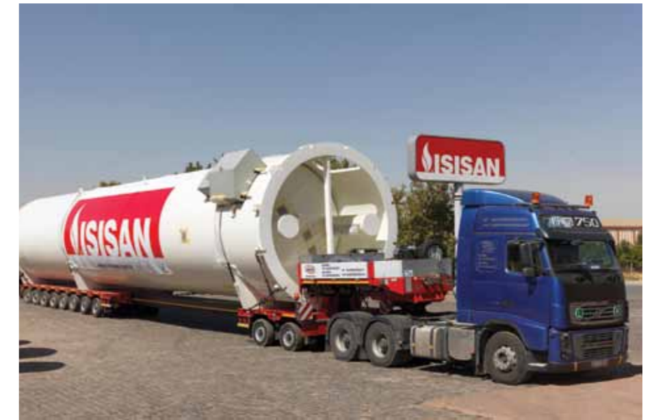
200m³ Cryogenic tank successfully supplied to Messer for an ASU plant located in Bor / Serbia
